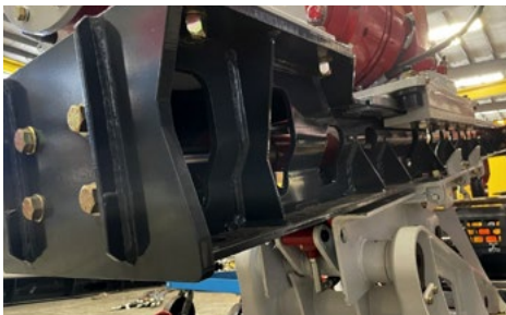
Engineered feed frame
