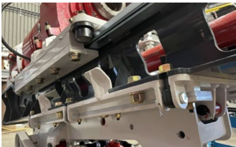
24" mast dump sub frame
