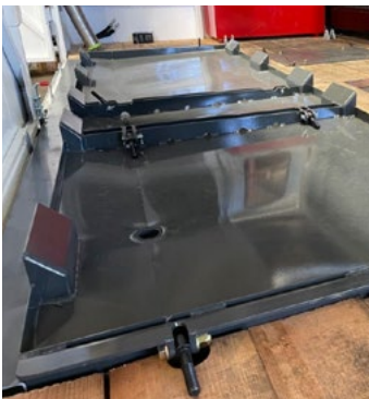
Integrated drill mounts & drip tray
