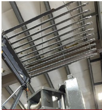
Rod handling and stacking system
